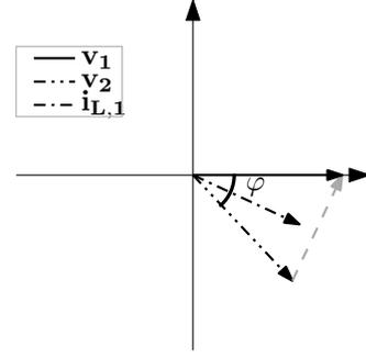
Fig. 5: Phasor diagram of the signals at fundamental frequency  $f_{sw}$ .
