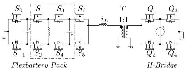
Fig. 1: An example of a single-unit Flexbattery H-Bridge converter. The basic Flexbattery unit is indicated in the dotted rectangular block.
