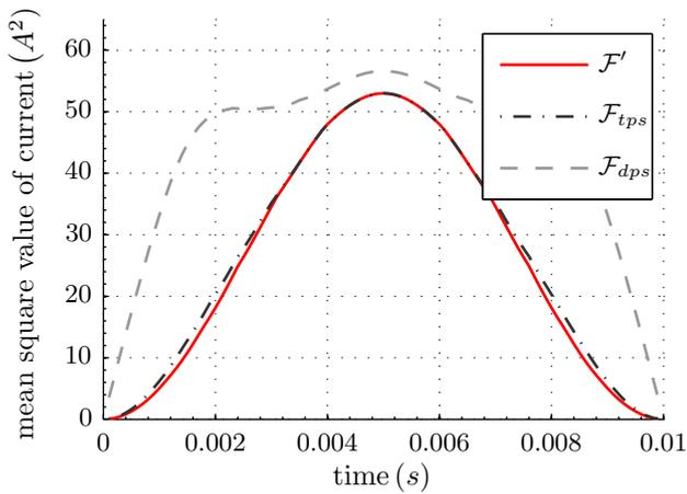
Fig. 11: Comparison of the proposed control method, TPS and DPS when  $Z_L = 0.5Z_{L,max}$ : results over half a grid period;
