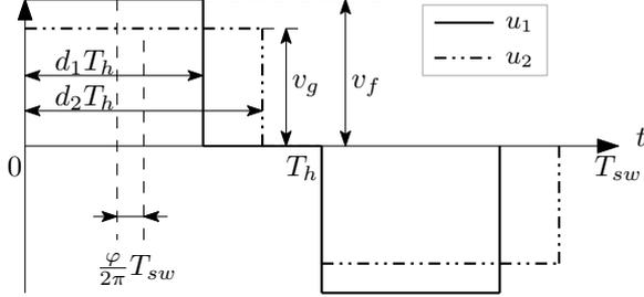
Fig. 4: Voltage waveforms for the proposed four-degree-of-freedom control method with four control variables  $v_f, d_1, d_2, \varphi$ .
