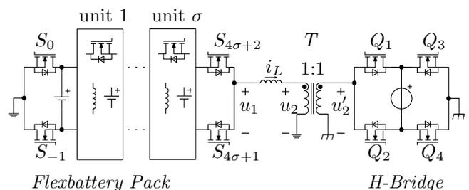
Fig. 2: General block diagram of the Flexbattery H-Bridge converter with  $\sigma$  extended commutation units.
