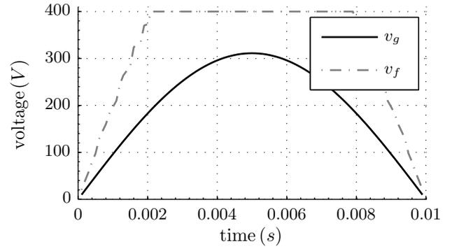
Fig. 7: Four-degree-of-freedom control optimization plot: voltages over half a grid period.
