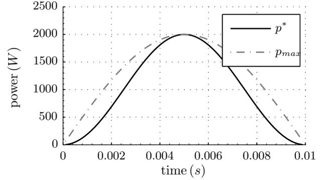
Fig. 6: The waveforms of the power set-point  $p^*$  and the maximum instantaneous power the converter can transfer  $p_{max}$ .
