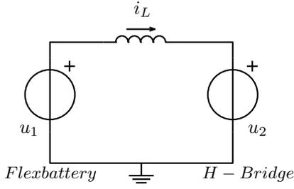
Fig. 3: Simplified circuit referred to the Flexbattery pack side.
