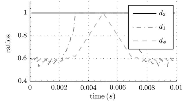
Fig. 8: Four-degree-of-freedom control optimization plot:  $d_1, d_2, d_\phi$  over half a grid period.
