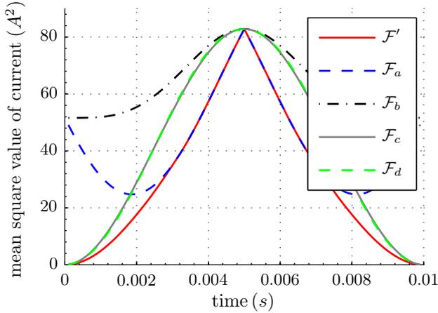
Fig. 9: The waveforms of the resulting mean square value of the current over half a grid period: solid red trace, proposed strategy; dashed blue trace, strategy *a*; dash-dot black trace, strategy *b*; solid grey trace, strategy *c*, dashed green trace, strategy *d*.
